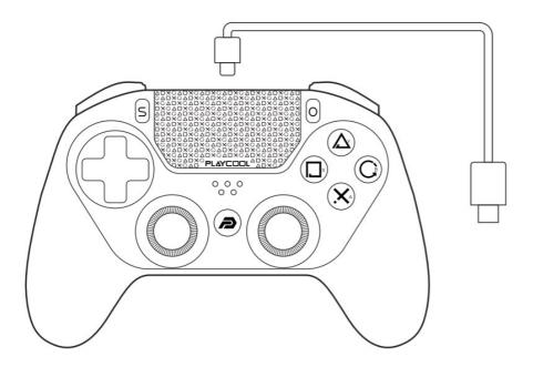
To a Type-C port on the PS4 system. Type-C cable (supplied in the gift box).
