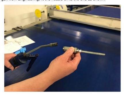
2. Lubricate the rail table bearings as shown below... Please avoid excess lubricant.
