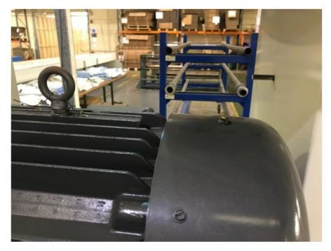
8. Lubricate nipples as shown of fan belt casing.
