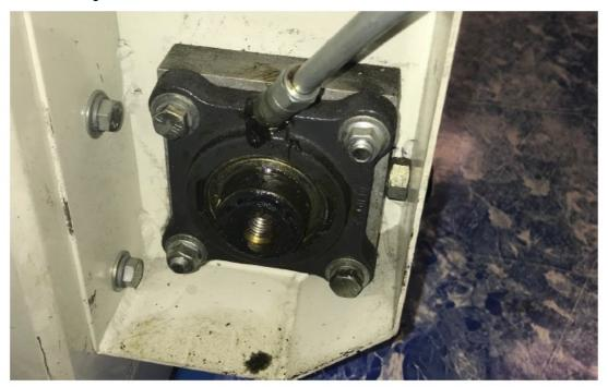
6. Check gantries for any debris or visible problems that will stop the tracks from moving.
