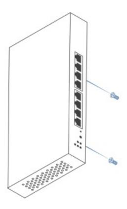
This Switch can be mounted either vertically or horizontally to a wall:
