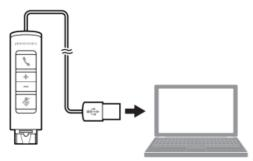
The USB Audio Processor is automatically powered on upon inserting into the USB port of the computer.
