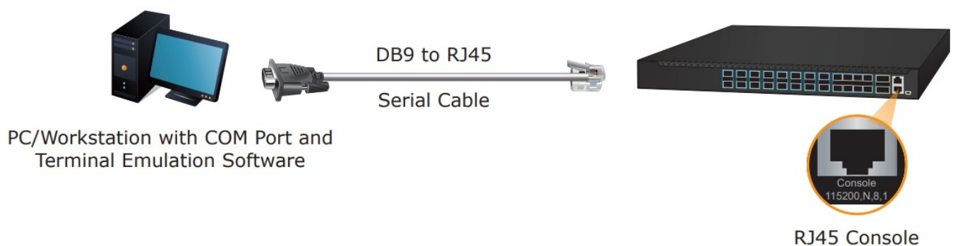
Figure 5-1: XGS-PON OLT Console Connectivity
