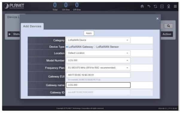
4. Set up the LoRaWAN gateway on the LCG-300 device.
