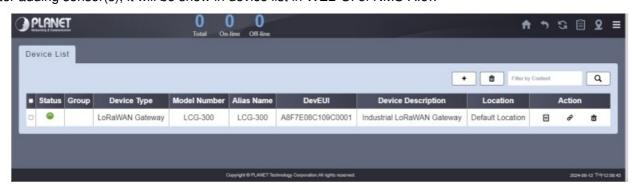
**Step 3:** Add new LoRaWAN sensors to the NMS-AloT system.
