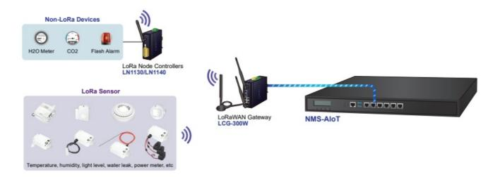
**Step 2:** Add a new LoRaWAN gateway to the NMS-AloT system, such as the LCG-300, LCG-300W, or LCG-300-NR.
