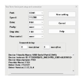
Figure 7-2: COM Port Configuration
