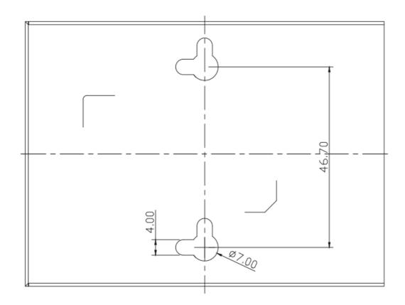
Step 3: Hang the LRE-101C on the screws from the wall.
