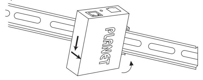
Step 3: Check whether the DIN rail is tightly on the track.
