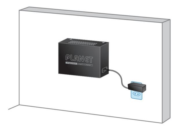
Before mounting the device to the wall, please check the location of the electrical outlet and the length of the Ethernet cable.
