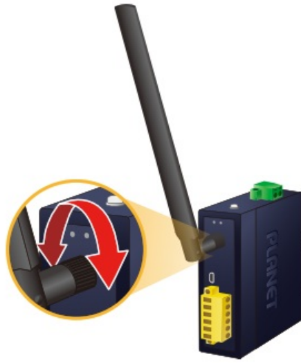
Figure 3: Connecting LoRa Antenna
