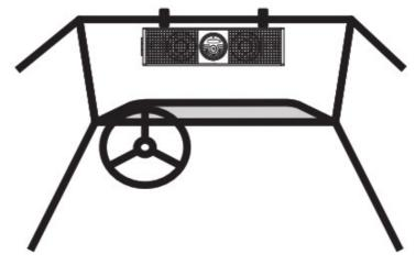
use the supplied adjustable bracket to secure to rails.
