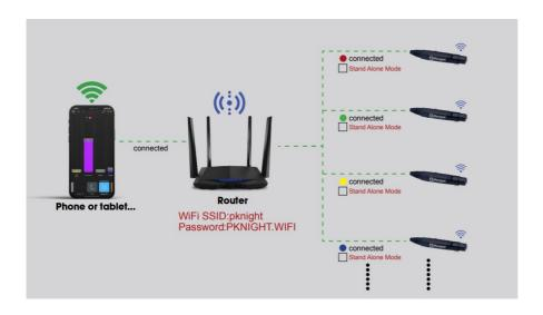
In router mode, we want to build such a local area network, our mobile phone or tablet computer and multiple controllers are connected to the 2.4G WiFi signal of the router. Buying a better router and assigning different wifi channel of controller will also optimize the stability and speed and range of the system's signal transmission.
