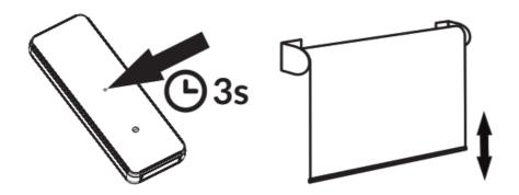
2. Press the CHANNEL + STOP buttons at the same time, the motor will move to confirm the operation.
