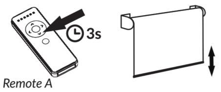
2. Using the new remote control (B), press the SET button on the back of the remote control, and the motor will move to confirm the new remote/channel was paired.
