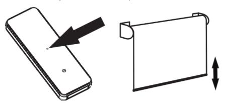
3. Press the SET button on the back of the remote control, and the motor will move to confirm that the new close limit position has been saved.
