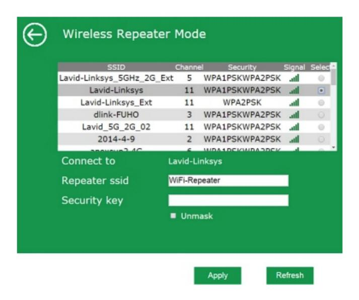
4. Click on "Apply" button, The W i-Fi Repeater will restart. After the reboot has been completed, the W i-Fi Repeater is accessible under the SSID and the Wireless key.
