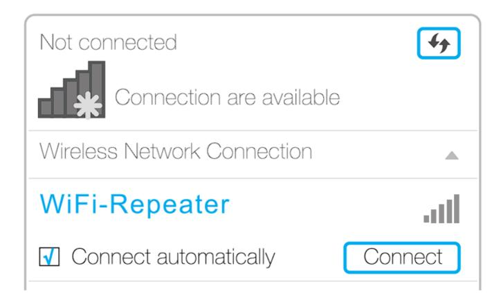
Disconnect your Ethernet (wired) connection from your computer. Click the W i- Fi icon on the taskbar and connect to the Repeater's network (e.g. WiFi-Repeater).
