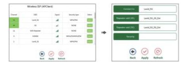
Select the SSID of the target network and insert Repeater SSID and the key of your network. the default Repeater SSID is set to be x0xx\_2G\_Ext/ xxxx\_5G\_Ext (xxxx indicates The Main Router's wireless network name). Then click Apply to complete setup.
