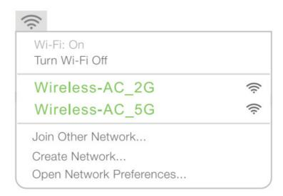
Disconnect the Ethernet (wired) connection from your computer (if any). Click the Wi-Fi icon in the top right corner of the screen, and connect to the Repeater's network (e.g Wireless-AC\_2G/5G)
