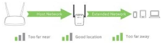
2. Wait until the signal LED displays two or three lattice signals.
