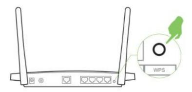
The WPS LED will be blink when pressing the WPS button, the xxXX\_2G\_Ext/xxxx\_5G\_Ext appear in your wireless network list, indicating a successful WPS connection,(XXXX indicates The Host Router's wireless network name). If not, please use Web Browser setup.
