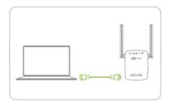
Disable the Wi-Fi on your computer. Connect your computer to the Repeater via an Ethernet cable
