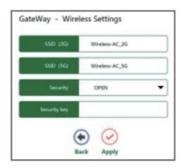
S510(2G)/S51D(5G)- Enter a value of up to 32 characters. The same name of 55/D (Service Set Identification) must be assigned to all wireless devices in your network. The default SSID is set to be Wireless-AC\_2G and Wireless-AC\_5G. Security you can choose the security type on the drop-down list. The default setting is OPEN. Security key – Wireless Password, When WPA/WPA2PSK is set as the Security Type, You can enter ASCII characters between 8 and 63 characters or 8 to 64 Hexadecimal characters.
