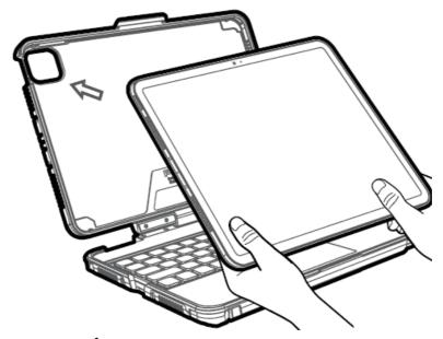
STEP 6: Press the corners of the iPad into the iPad shell, beginning with the camera and button. The iPad will snap securely into the case's perimeter seal. Reference STEP 1 if necessary.
