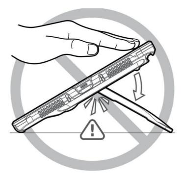
Do not attempt to force the PIVOT Kickstand beyond the maximum 120-degrees of rotation or adjust the Legs independently. Doing so may result in damage to the Kickstand, hinges, and case body.
