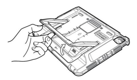
Locate the Center Finger Tab and lift gently. Apply constant force while lifting to disengage the two Snap-Closures, which are located to the left and right of the Center Finger Tab. An audible "Click" may be heard as the closures release.
