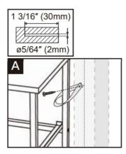
• For Concrete or Solid Wall Installation
