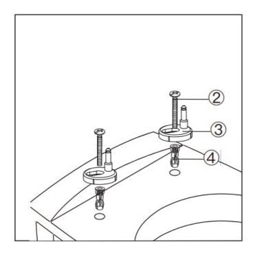
• Untighten the screws a bit by turning them 90° in a anti-clockwise direction. This will allow you to align the seat
