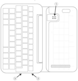
Open and place the keyboard flat on a hard surface with the hinge fully extended. Proceed to insert the PinePhone into the keyboard at an angle of approx. 15 degrees. Make sure that the PinePhone's pogo pins and the corresponding pads on the keyboard are aligned. The leading edge with volume and power buttons should make contact first. Firmly press the PinePhone into place. Multiple clicks should be heard as the two snap into place.
