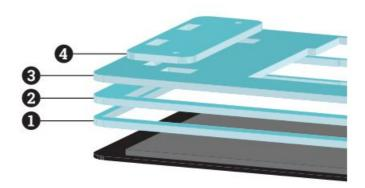
Place your Raspberry Pi 7" Touchscreen Display face down on a soft non-scratch surface and lay frames (1, 2, and 3) on top of it.
