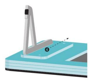
Slide the locking stand plate upwards which will align the screw holes through to the display's metal bracket.
