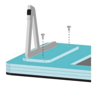
Screw in the four M3 nylon bolts until the stands are firmly secured. Don't overtighten them!
