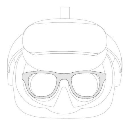
**Install Glasses Spacer:** If you have glasses collision with headset lens or pres-sure on the bridge of nose, please follow the picture to install Glasses Spacer to increase the space. You can install or not according to your situation.
