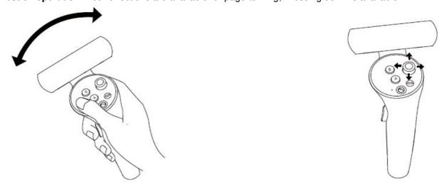
**Switch the pointer of the master Controller:** In the home screen, short press the TRIGGER button of the corresponding Controller to switch the pointer of the master Controller.
