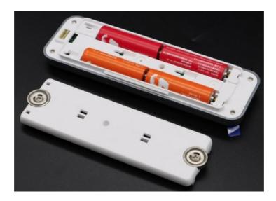
1. AA\*4 battery pack power supply (Battery version
