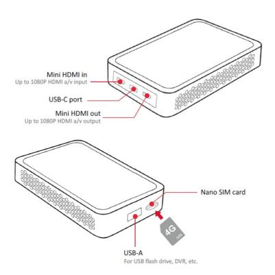
**NOTE!** Power off before inserting or removing the nano SIM card. Nano SIM card is not included in the package. For how to insert the card please refer to this diagram.
