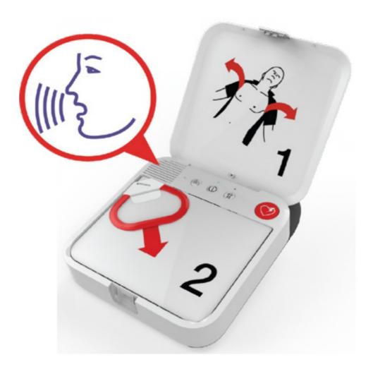
**c.** Immediately press and hold the LANGUAGE and CHILD MODE buttons simultaneously until you hear "Device ready."
