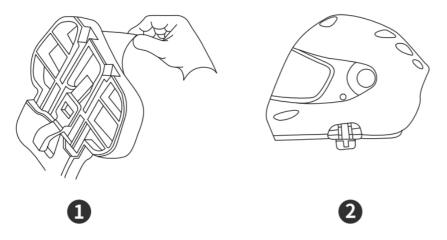
Tear off the rough surface of the left and right speaker Velcro on the headset, and paste them on the left and right ears of the helmet, then After attaching the speaker to the Velcro surface in the helmet, the speaker with short headphone cable is installed in the left ear.
