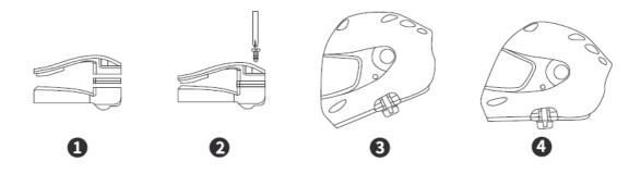
If there are any problems with mounting the bracket, you may use the 3M tape bracket .peel off the protective backing sheet of the 3M tape and adhere the bracket onto the helmet.Pressfor15 seconds and glue dry for 24 hours.
