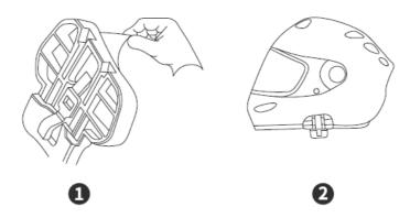
Tear off the rough surface of the left and right speaker Velcro on the headset, and paste them on the left and right ears of the helmet, then After attaching the speaker to the Velcro surface in the helmet, the speaker with short headphone cable is installed in the left ear.
