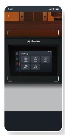
4. Scan the QR code provided on your 3D printer screen to bind your account, then confirm the connection on the 3D printer screen.
