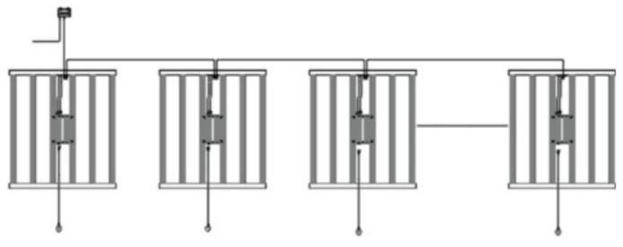
**NOTE!** Each of the controller's two channels (Zone A & Zone B) can control up to 50 LED fixtures. It is possible to use those channels to control LED fixtures in two separate rooms or to control up to 100 fixtures in one room.
