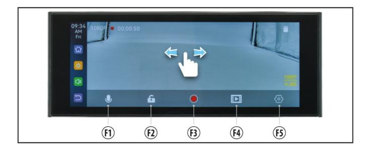
The screen opens on the front video camera; scroll to display the rear-view camera. The display keeps the last position in memory.
