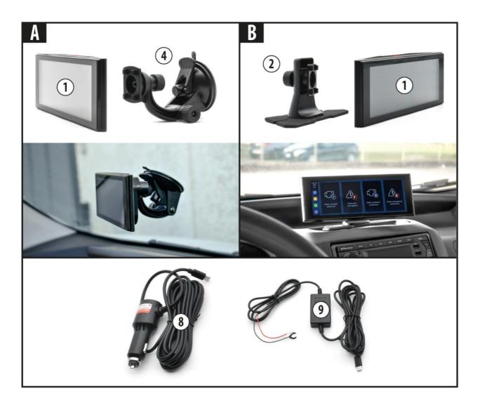
N.B. Identify the installation position for the display: this must not obstruct the driver's view or the operation of safety devices, and must not inhibit the freedom of movement required for safe driving.
