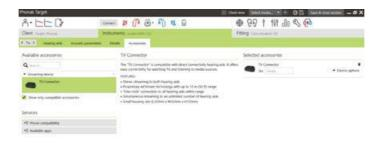
Depending on the connected hearing aids, Phonak Target can automatically identify connected accessories during the fitting session. The compatible accessories are shown in the dashboard next to the connected hearing aids.
