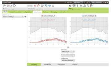
Depending on the connected hearing aids, additional tools such as [Tinnitus Balance] and [CROS Balance] can be accessed via the tab in the lower part of the screen. To adjust the loudness ratio between the CROS device and the hearing aid, click on [CROS Balance].
