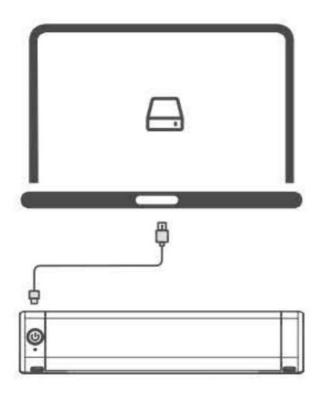
Connect the printer to your computer with a Type-C data cable
