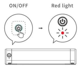
Press and hold for 3s to turn on the MOSF printer
