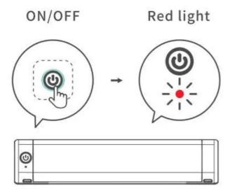
Press and hold for 3s to turn on the MO8F printer
