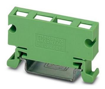
Press-drawn section housings, Lateral element, color: green (6021), with snap-on foot, depth: 45 mm, Note: when using this lateral element, profile length = PCB length.
