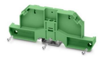
Lateral element, to attach profile cover UM 122 to DIN rail NS 35/7.5, with M3 screw fixture, tightening torque 0.25 Nm
