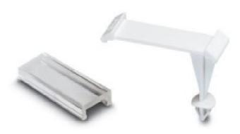
Phoenix module marker carrier, for labeling modules and PCBs, for hole diameter 3.9 to 4.1 mm, thickness of wall or board 1.5-2.0 mm, labeling with insert strips ESL, EST or ES/LP-BW-GB, lettering field:  $29 \times 8$  mm
