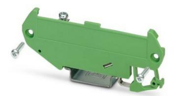
Side element, left, with foot, width: 5 mm, length: 72 mm, for mounting on NS 32 or NS 35/7.5, with PE contact to the DIN rail
