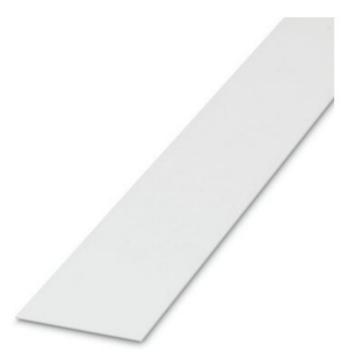
Insert strip, white, unlabeled, mounting type: insert, for terminal block width: 35 mm, lettering field size:  $35 \times 500 \text{ mm}$
