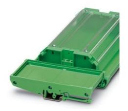
Press-drawn section housings, Basic profile, open, length: 2000 mm, cross connection: without bus connector, color: green, Note: profile length = PCB length - 3 mm (UM 25 and UM 45) Profile length = PCB length - 3.6 mm (UM\_72, UM 100, UM\_108) Profile length = PCB length - 9.5 mm (UM\_122)
