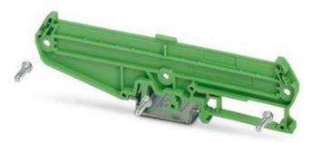
Side element with foot, 5 mm wide (right), for mounting on NS 32 or NS 35/7.5. PCB width: 107.5 mm **Lateral element**
