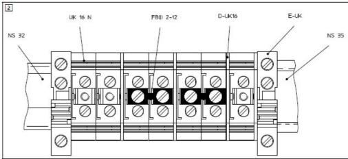
Feed-through terminal block with screw connection for use in potentially explosive areas The terminal is designed for connecting and linking copper wires in wiring spaces with "eb", "ec" or "nA" types of protection.
