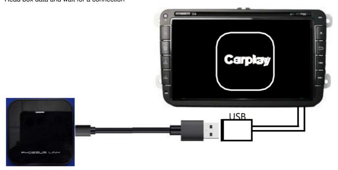
2. Turn on the Bluetooth of the iPhone, search for the Bluetooth Device naming: "smart Box-\*\*\*\*". Pair it and allow the Sync, finally click "Use Carp lay
