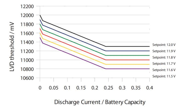
**Mode 2 voltage:** Load disconnect level can be set between 11.0/22.0 V and 11.5/23.0 V. It is appropriate if bypass loads draw current directly from the battery. This mode allows a lower disconnection point. The battery is cycled deeper, and this can shorten battery lifetime.
