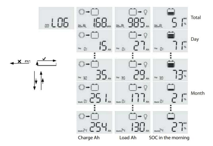
The CXNup controller has a 2 years datalogger. Push the "ESC" (X) button when the LCD is scrolling the current values and the controller will enter the menu. Select "LOG" with the arrow keys and press "SET" () to enter the datalogger menu. You can get the charge Ah, load Ah and SOC in the morning, as daily data for a month, monthly data for two years and total data.
