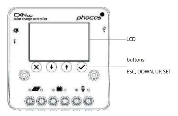
In normal operation, the controller shows the state of charge of the battery and the solar panel activity. Any change of the state of charge (SOC) to a lower status is additionally signaled acoustically.
