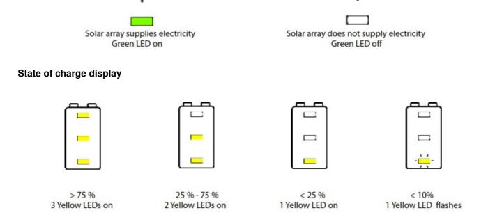
The percentage corresponds to the available energy until Low Voltage Disconnect with respect to a fully charged battery.
