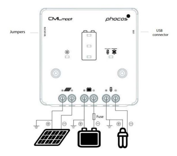
connecting a fuse directly to the battery to protect any short circuit at the battery wiring. The fuse must correspond to the nominal current of the charge controller: 15A for CMLmppt 10.
