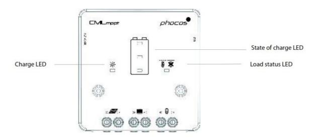
In normal operation, the controller shows the state of charge of the battery and the solar panel activity. Any change of the state of charge (SOC) to a lower status is additionally signaled acoustically.
