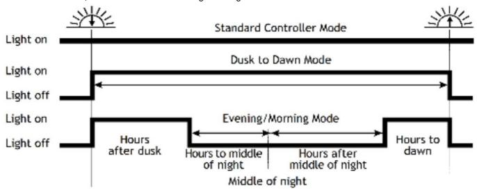
"Middle of night" is detected automatically as the midpoint between dusk and dawn, no setting of a clock is required. It may take several days until the controller has "learned" the middle of the night precisely. "Middle of night" may be different from 12:00 midnight depending on your location.
