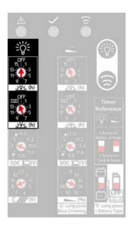
In column 2, change "Evening (h)" to 15, and change "Morning (h)" to 14. (Note that the D2D setting only applies to dual load CIS controllers, not to dimming settings.) Do not worry about the numbers being longer than the actual night length. The controller will still intelligently detect dusk and dawn based on PV voltage.
