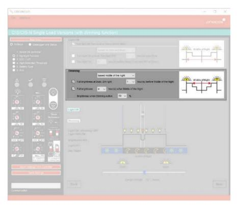
5. In the Dimming menu section, change the hours dropdowns to their maximum values. Do not worry about the numbers being longer than the actual night length. The controller will still intelligently detect dusk and dawn based on PV voltage.
