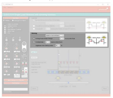
4. In the Dimming menu section, change the dropdown option from "based on dusk and dawn" to "based middle of the night".
