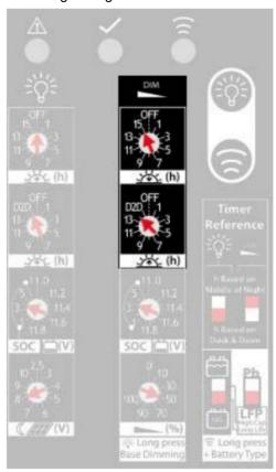
In the Timer Reference area, select "h based on Dusk & Dawn" for Timer Reference 1, and select "h based on middle of night" for Timer Reference 2.
