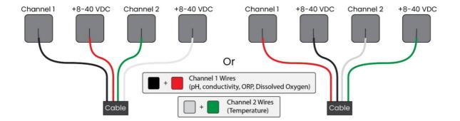
D-phi Series<sup>™</sup> sensors have Reversible Input Protection (RIP). This means that the red and black wires function interchangeably as the power and output. RIP prevents damage occurring to the receiver or sensor due to improper wiring and simplifies the wiring process.
