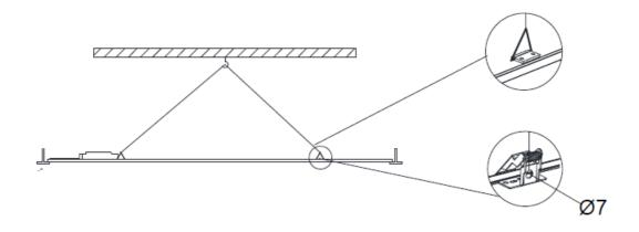
The product (include two mounting types) should install safety chain (Safety chain is not included in package.).
