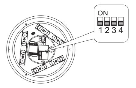
Detection area (default 50%) Detection area can be increased by selecting 100% on the DIP switches to fit precisely each application.
