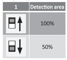
Hold time (default 3 min.) Refers to the time period the lamp remains at 100% illumination after no motion detected.
