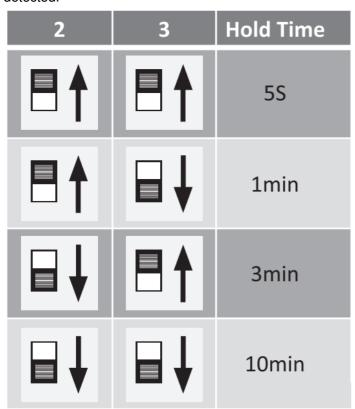
Daylight sensor (default enable mode) The sensor can be set to only allow the lamp to illuminate bellow a defined ambient brightness threshold (251ux). When set to disable mode, the daylight sensor will switch on the lamp when motion detected regardless of ambient light.
