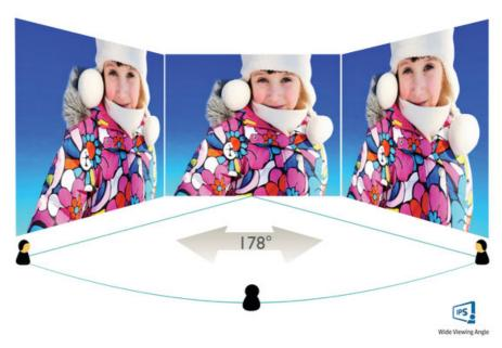
IPS displays use advanced technology which gives you extra-wide viewing angles of 178/178 degree, making it possible to view the display from almost any angle – even in 90-degree Pivot mode! Unlike standard TN panels, IPS displays gives you remarkably crisp images with vivid colors, making it ideal not only for Photos, movies and web browsing but also for professional applications which demand color accuracy and consistent brightness at all times.
