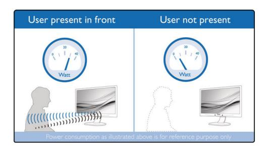
PowerSensor is a built-in 'people sensor' that transmits and receives harmless infrared signals to determine if user is present and automatically reduces monitor brightness when then user steps away from the desk, cutting energy costs by up to 70 percent and prolonging monitor life.
