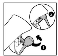
This side docking allows you to access steamer head conveniently without the hassle of reaching high up. You can choose to use the side docking at either the right side or left side of the device.
