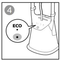
The power button flashes indicating that the appliance is heating up. When the appliance is ready for use after 90 seconds, the light turns steady.
