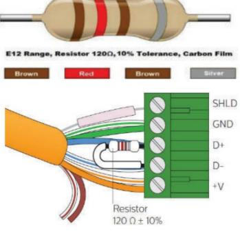
8. The maximum recommended length for DyNet cables between two network bridges is 800 m (2620 ft). For cable runs over 300 m (1000 ft), (or baud rates over 9600 bps), 120 Ohm, 2 W end-of-line resistors must be installed across the D+ and D- terminals of the DyNet connector strip on the first and last devices.
