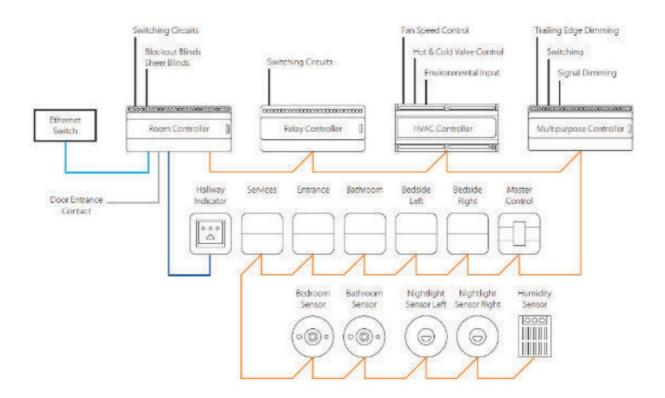
1. The data cable is connected to all devices as per the project schematic following the correct color code and DyNet terminations. Devices may be wired in any order.
