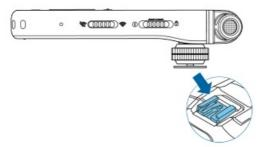
3. Use both adjusting screws on the hot shoe adapter to ensure that your VoiceTracer is fixated on your video
