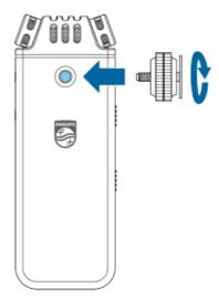
Slip the hot shoe adapter into your camera's hot shoe. Make sure to direct the front of your VoiceTracer in the direction you want to record.
