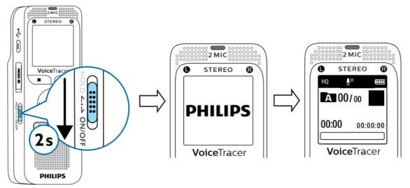
Slide the on/off switch on the side of the device down for two seconds
