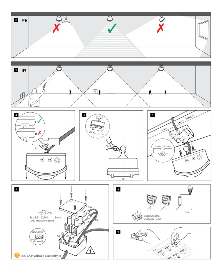
Do not connect inputs to mains. DALI wires are NOT SELV and should never be considered touch safe.
