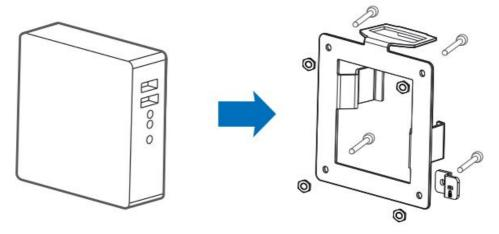
3. Slide down the bracket with the mounted device into the Philips Height Adjustment base.
