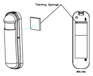
After finish the test and decide to fix, then you can remove tape A, and mounting the sensor by using tape B. The tamper key will be pressed and let the sensor normal mode.
