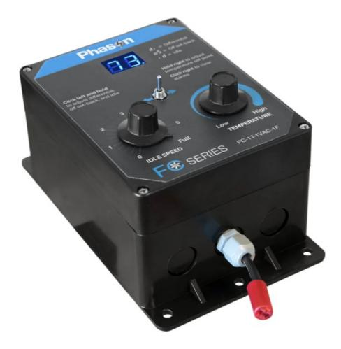
The FC-1T-1VAC automatically controls ventilation fans according to temperature. When the temperature is at the set point, the control operates the fans at the idle speed setting. When the temperature exceeds the set point, it increases the speed of the fans. The FC-1T-1VAC has two modes of operation:
